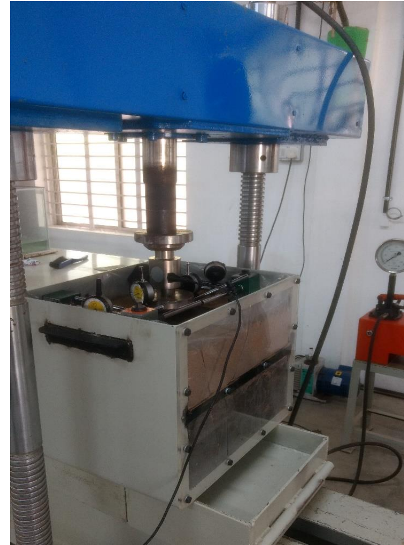
Model Footing Test Setup Fabricated
