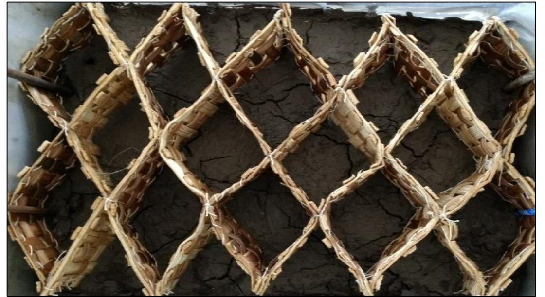
Areca cell reinforced clay bed
