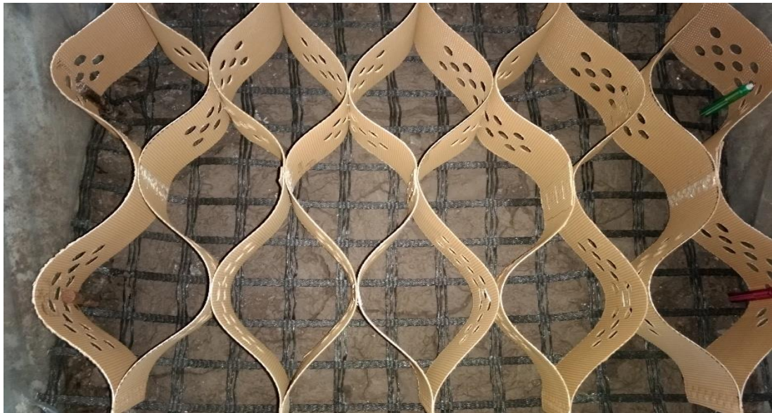
Geocell + Geogrid reinforced clay bed
