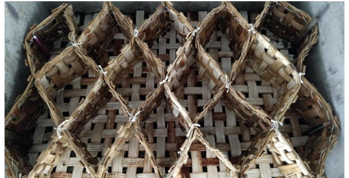
Areca cell + Areca grid reinforced clay bed
